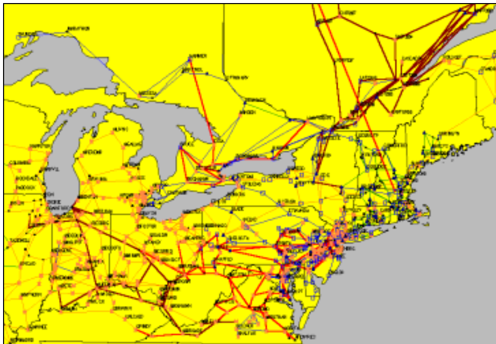
Figure 4. Transmission Line Network for Eastern Interconnect
